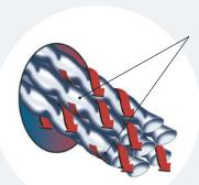
UNIFORM SHELL SIDE **VELOCITY CAN REDUCE** FOULING CAUSED BY DEAD SPOTS.
