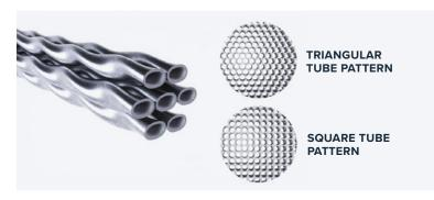
The "twisted" baffle-free arrangement of the tubes provides gaps that facilitate convenient cleaning on the shell side while the round ends of the tubes allow for the use of conventional tube-to-tubesheet joints. Both the profile of the individual tubes and the width of the connection points between tubes can be varied to elongate cleaning lanes, further accommodating routine maintenance.
